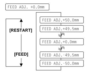
**[FEED]** key: Pressing the **[FEED]** key one time causes a -0.5mm change, up to -50.0 mm.
